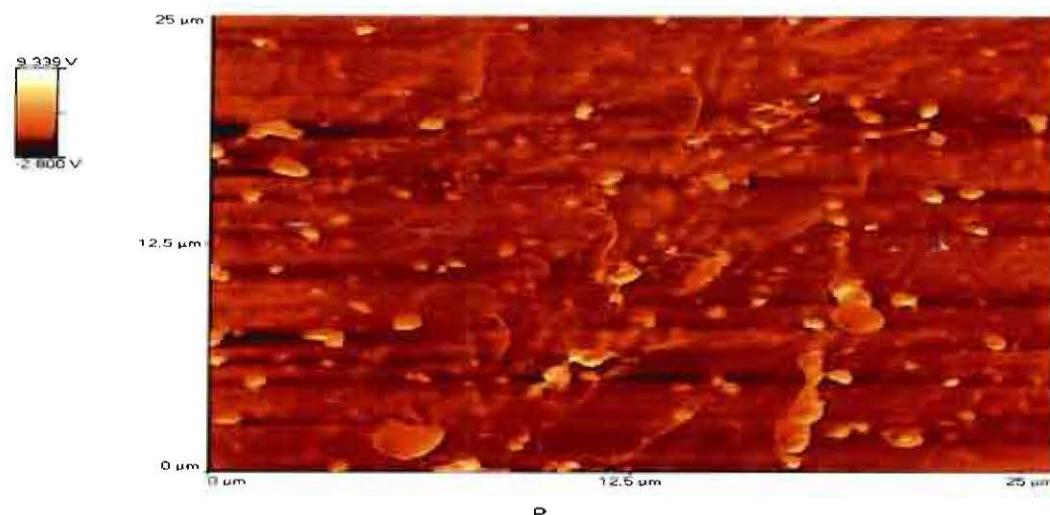
Fig 2.19: AFM image of nanocellulose reinforced polyethylene film
