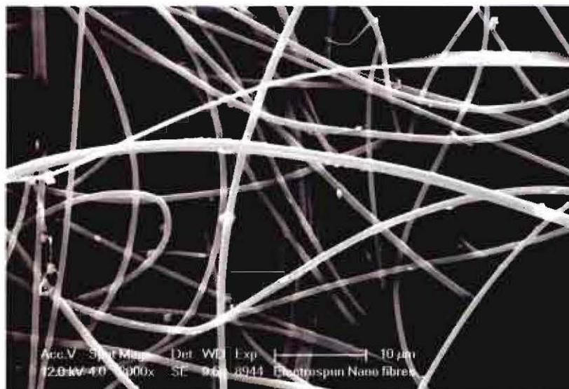
**Fig 2.11: SEM Image of electrospun fibres.**
