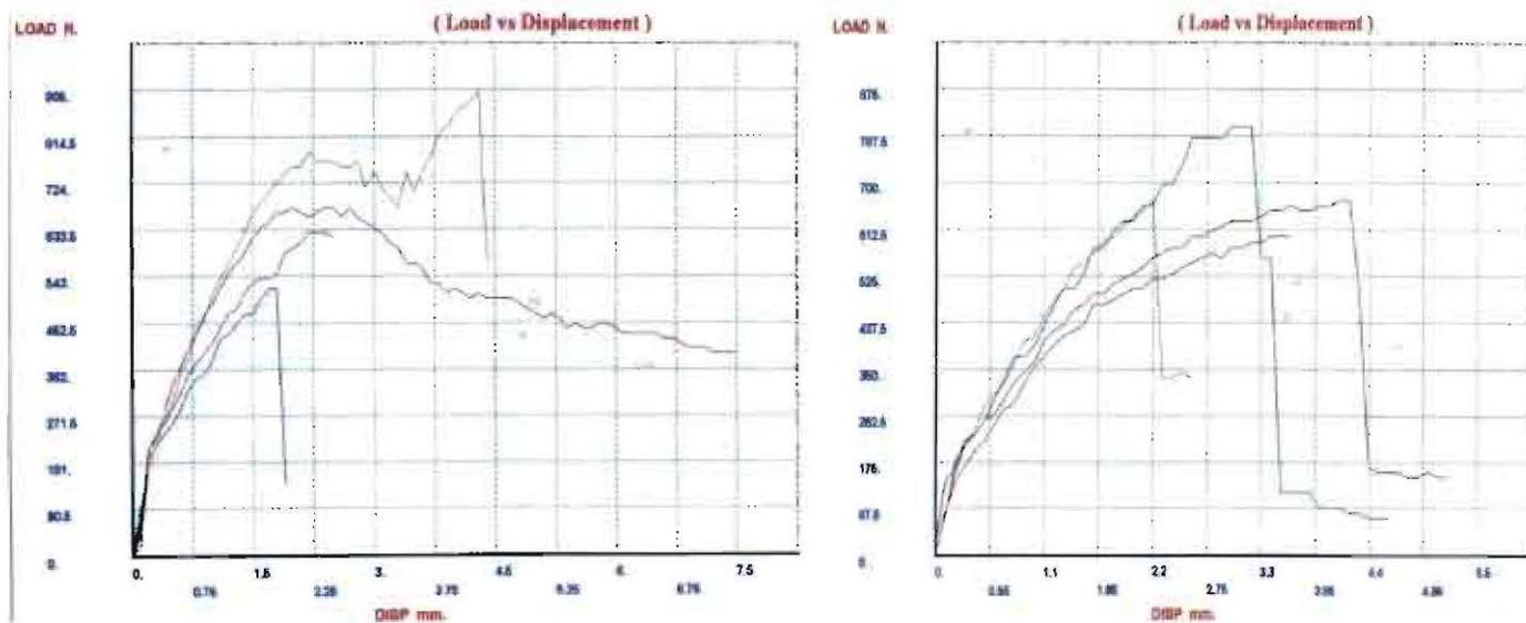
Tensile graph of Banana-polypropylene composite
