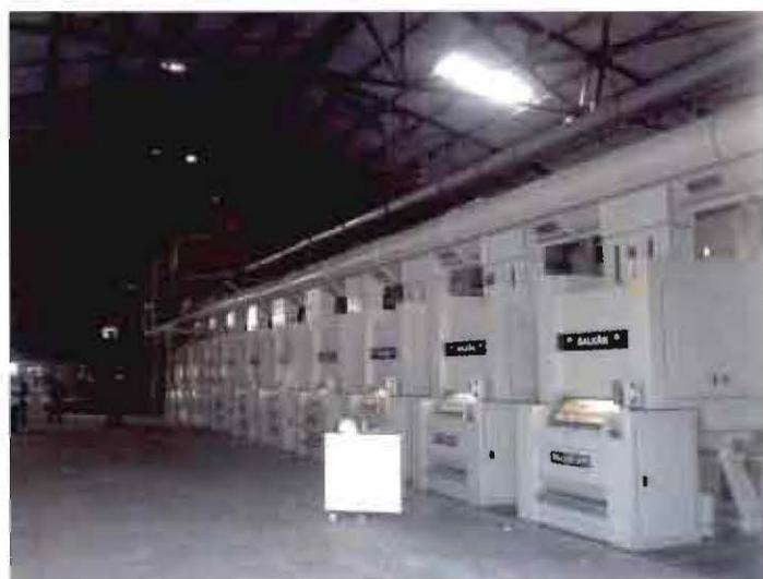
Fig. 2.4: Rotary Knife Roller Gin Plant
