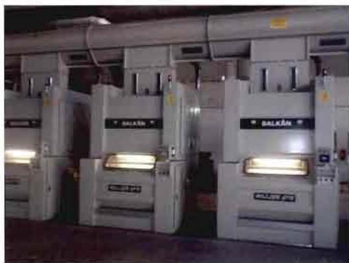
Fig. 2.3: Rotary Knife Roller Gin
