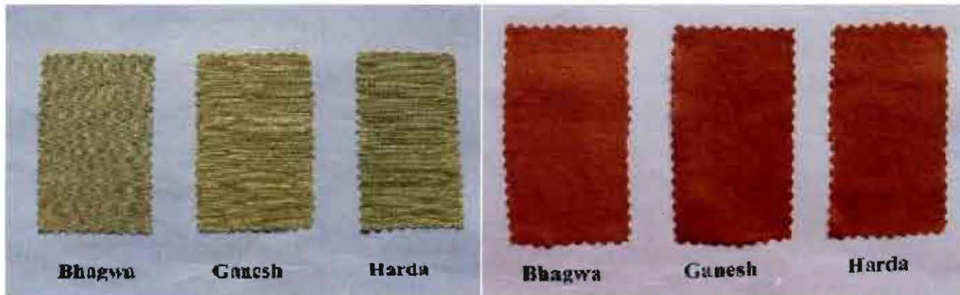
Fig. 2.18: Cotton fabrics mordanted with pomegranate rind powder and dyed to deep orange-red colour
