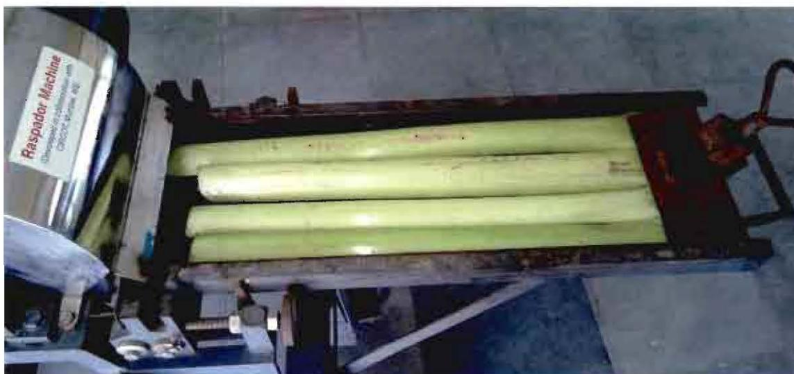
**Fig. 2.14: Multisheath feeder attachment on Raspador**
