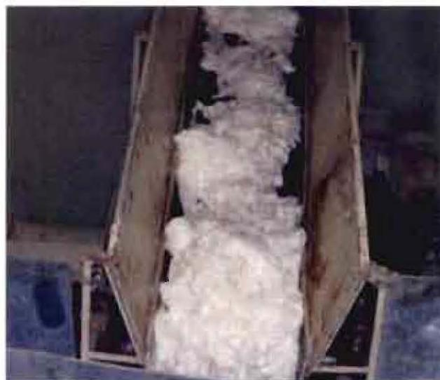
**Fig. 2.2: Uncovered belt type lint conveyors**
