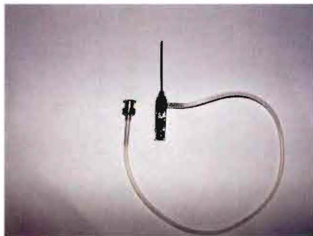
**Fig 2.10: Coaxial Needle**
