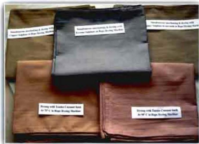
**Fig. 2.17 (a): Samples Dyed in Rope Dyeing machine**
